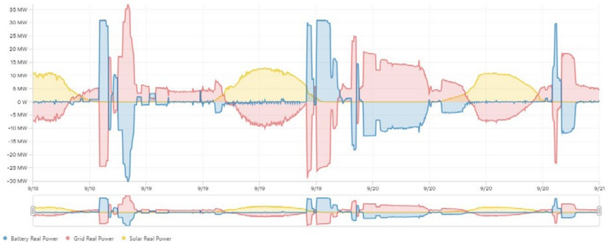
Figure 3-11. Load effects from battery real power (in blue), grid real power (in pink), and solar real power (in yellow), across a three-day span in Vermont, in MW.
