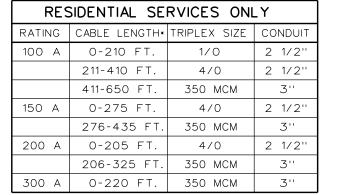
Cable Length is the total of trench and riser lengths.
